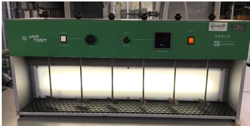
Figure 4.2 – Photograph of the jar-test apparatus, at FEUP.
