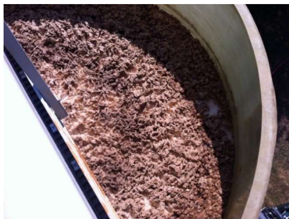
Figure 6.3 – Foam with sludge at the C/P unit surface (coagulation/sedimentation stage).
