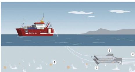
1. Scallops and clams are harvested using dredges 2. Steel teeth comb through the sea bed 3. Fins direct the dredge 4. Dredges can cause damage to sea floor habitats.
