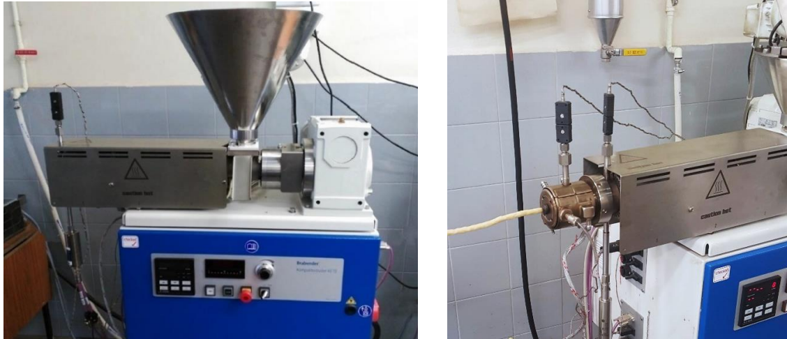
Figure 11. Single screw laboratory extruder turned off (left) and during the extrusion of corn and house cricket snacks (right).
