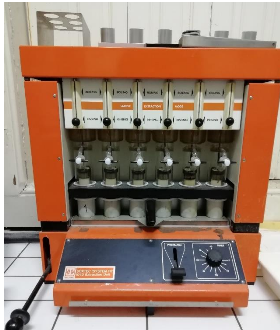
Figure 7 - SoxTec system, used to determine lipid content.
