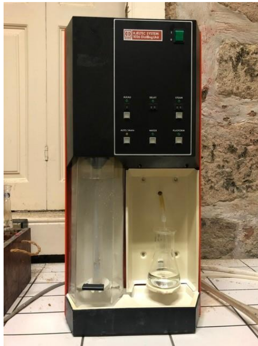
Figure 6 - Kjeltec distillation unit, used in the determination of protein content.
