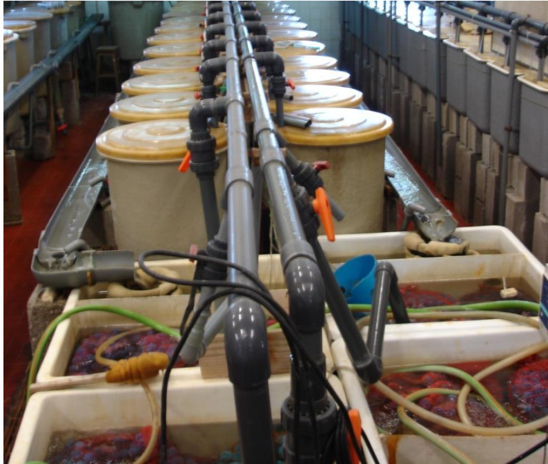
Figure 5 - Thermo-regulated recirculating water systems. The right side corresponds to the system subjected to thermal chronic stress and the left side to no thermal stress.
