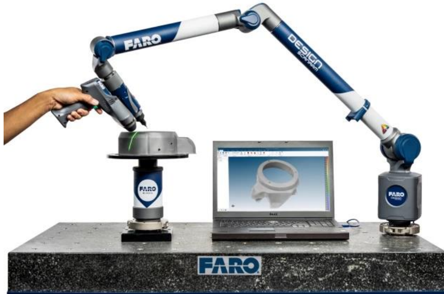
Figure 26 - Representation of the Metrology FARO solution used in this study. Gage Arm and Prizm LLP, CAM2, with the sample/prototype being attached to a marble table (courtesy of FARO® Technologies).
