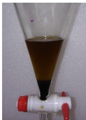
Figure 7.11. Separation of pre-treated oil (upper layer) after glycerolysis.
