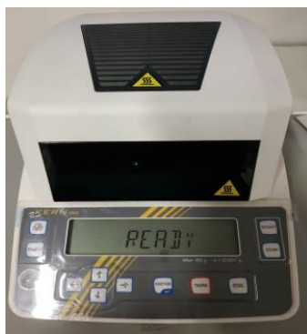
Figure 5.5. Infrared balance for automatic determination of moisture content determination.
