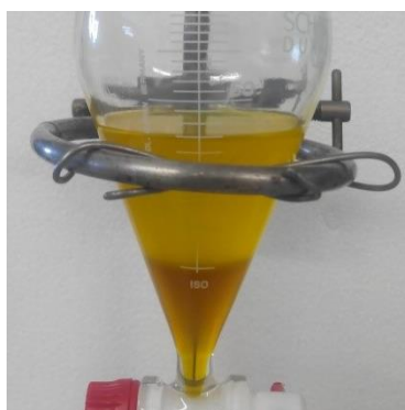
Figure 3.18. Biodiesel and glycerol obtained using refined crambe oil.
