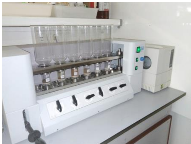
Figure 5.9. Vacuum system used for sample filtration aiming fiber determination.
