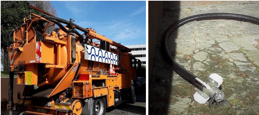
Figure 7: Mechanical rodding tank truck (left) and equipment for removing tree roots (right) used in AdP (Águas do Porto E.M. 2020)
