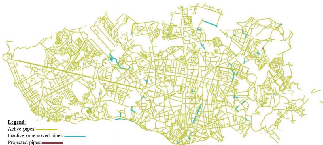
Figure 11: Drainage pipes of Porto's domestic wastewater drainage network (Águas do Porto E.M. 2015)
