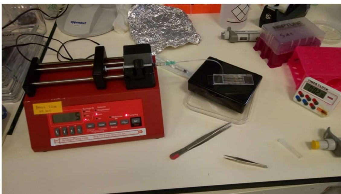
Figure A8 – Setup for the injection of the different solutions in the optofluidic chip for analysis. A syringe connected to a pump by an EVA tube was used for each injection. Each injection was made at a flow rate of 5 \mu L/min for 5 minutes, so the volume injected was 25 \mu L for every case.
