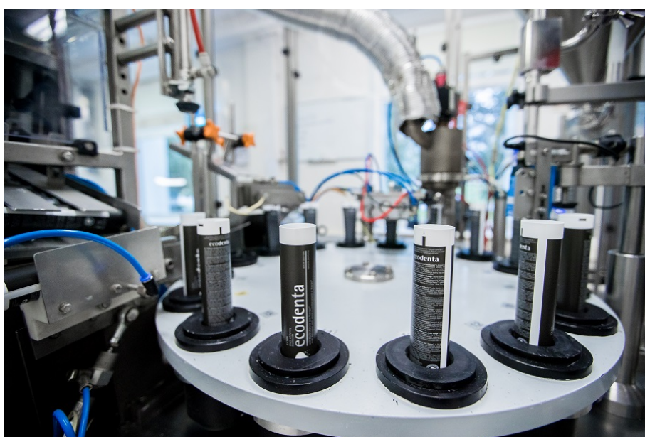
Figure 2: Production line at the BLOK factory facilities, depicting the loading of toothpaste tubes onto the filling machine (134).
