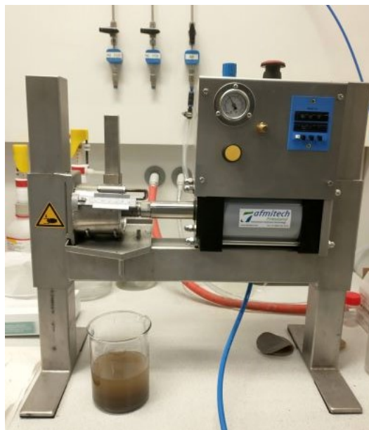
Figure A.5: Press filter Setup: Includes a manual lever that allows for faster or slower pressure
