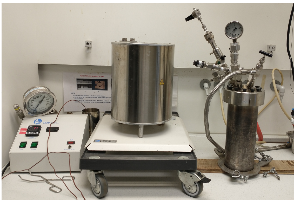
Figure A.1: THP Setup: Includes a temperature PDI controller, a heat isolated chamber and a insert where the samples are placed within.
