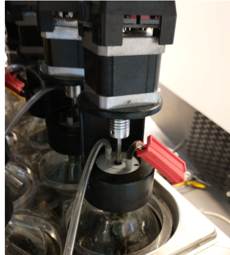
Figure A.3: Cap of a test bottle with 3 inserts: the rotator, the tubing for CH 4 measurement and the sampling point with a red clamp to ensure anaerobic conditions.
