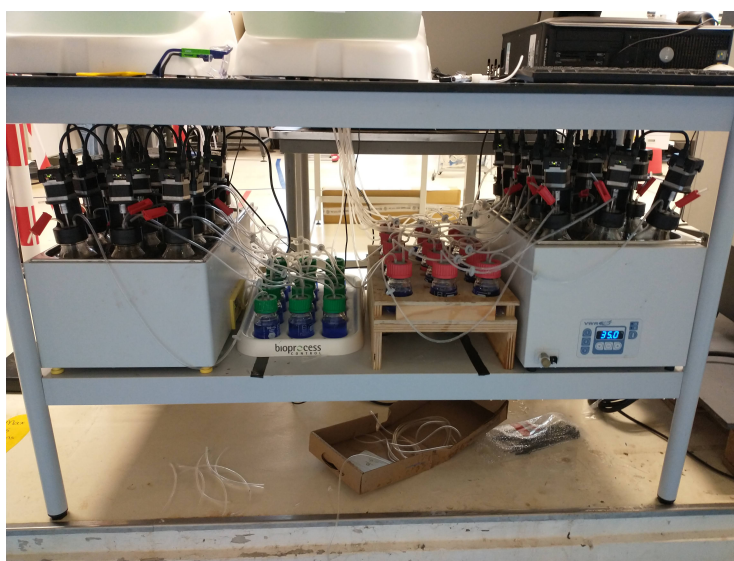
Figure A.2: BMP setup. The sample incubation unit (unit A) and the CO 2 -absorbing unit (unit B) are shown in the forefront. On top of the working bench, unit C is also slightly displayed.
