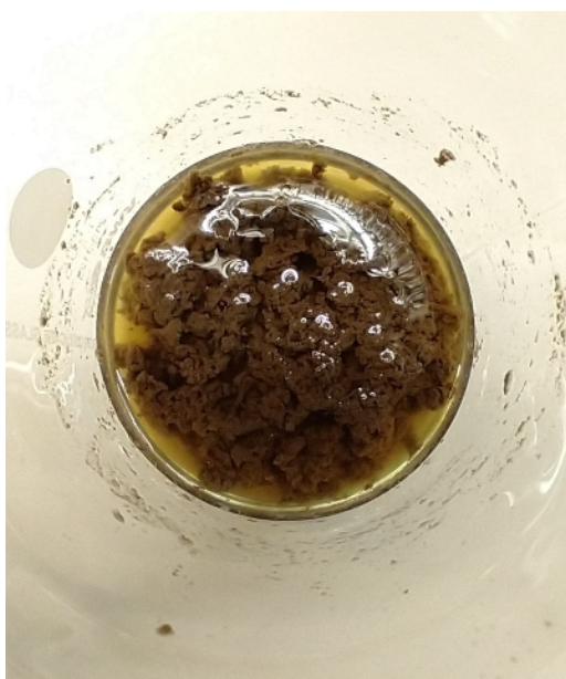
(a) Dewatering mixture with digestate and polymer.
