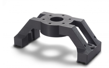
(b) FDM built nylon part [11]
