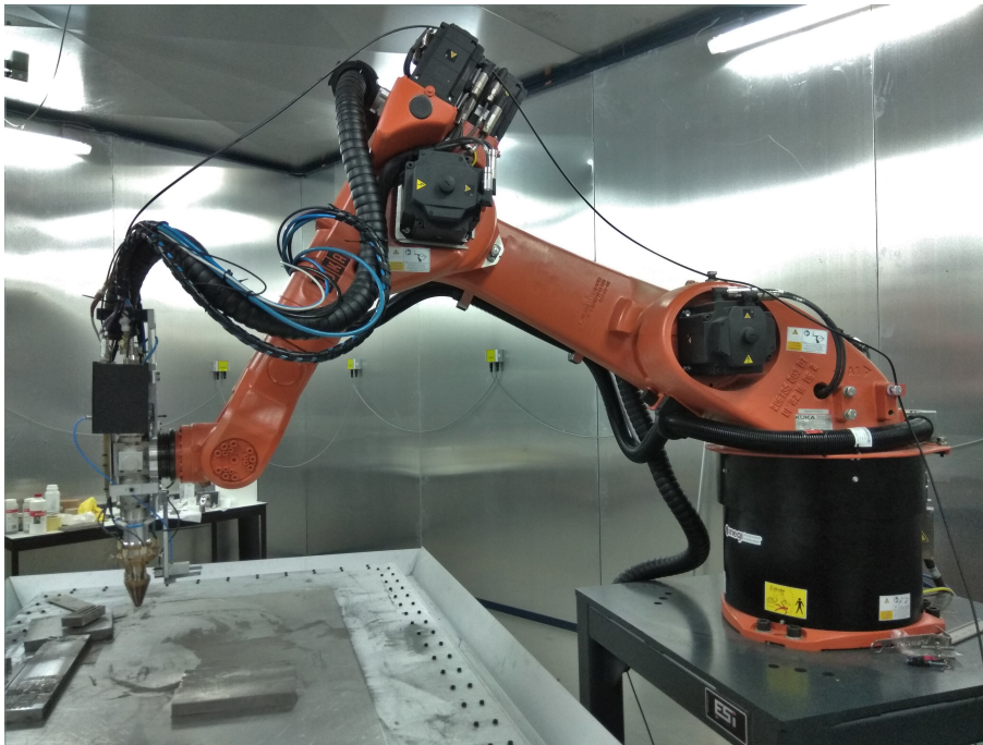
Figure 3.6: DED setup used
