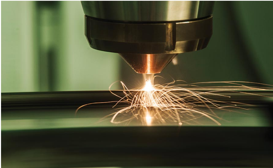
Figure 1.1: Direct Energy Deposition process with a coaxial nozzle [4]
