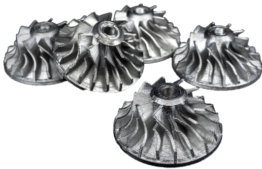
(a) BPE build metal parts [9]
