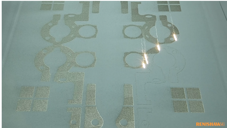
Figure 2.11: Lasers scanning the powder bed in a Renishaw machine [33]
