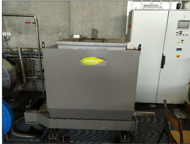
Figure 4.8 - The gasification plant's feed hopper, with the hatch closed.
