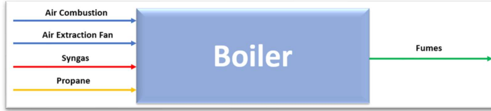
Figure 6.2 - Components entering and exiting the boiler.
