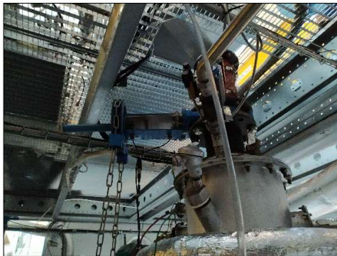
Figure 4.27 - Top of gasifier, with connection to the feed hopper (left). Various air insertions into the gasifier, as well as regulators and sensors (right).
