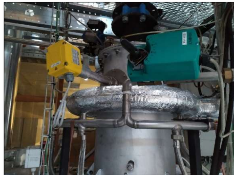
Figure 4.27 - Top of gasifier, with connection to the feed hopper (left). Various air insertions into the gasifier, as well as regulators and sensors (right).
