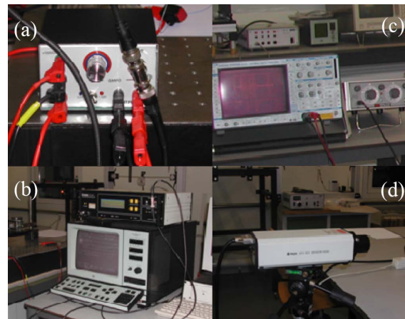
Figure 9.7: Equipment utilized: (a) operational amplifier; (b) dynamic signal analyzer Brüel & Kjær - 2035 and laser vibrometer controller Polytec - OFV 3001; (c) Digital oscilloscope LeCroy - 9450A and filter Krohn-Hite - 3550; (d) laser vibrometer measurement unit Polytec - OFV 303.
