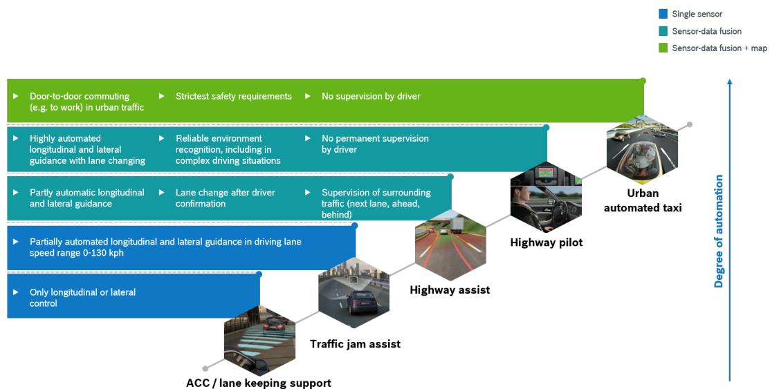
Figure 2.3: Automation steps for autonomous driving [6].
