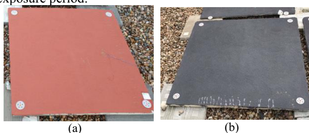
Fig. 3. Exposure condition: (a) Red specimen without nanopigments; (b) Black specimen without nanopigments.
