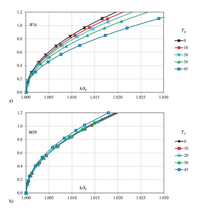
Figure 3. LCO amplitudes W/h against different aerodynamic pressures  $\lambda$ , for VSCLs with various fiber angle parameters; a) change of  $T_0$  ( $T_1 = 0^\circ$ ), and b) change of  $T_1$  ( $T_0 = 0^\circ$ ).
