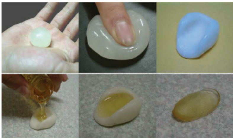
Figure 3.12: Artificial fingerprint molding process. From Marasco et al. (2014) [51].
