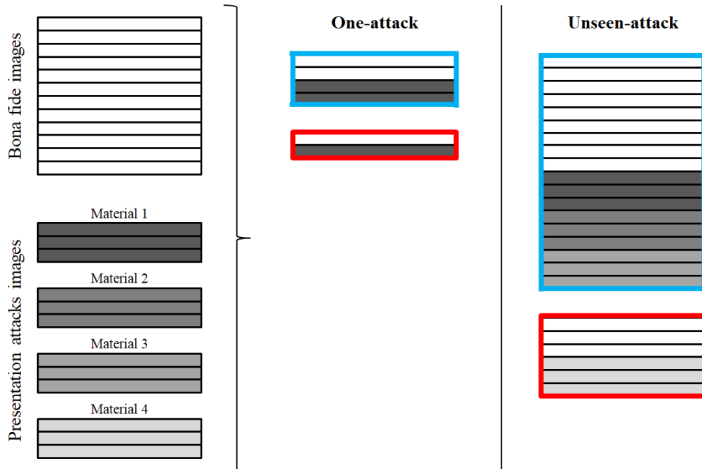
Figure 5.2: Frameworks: One-Attack and Unseen-Attack. The train/validation and test data are represented by blue and red limits, respectively.
