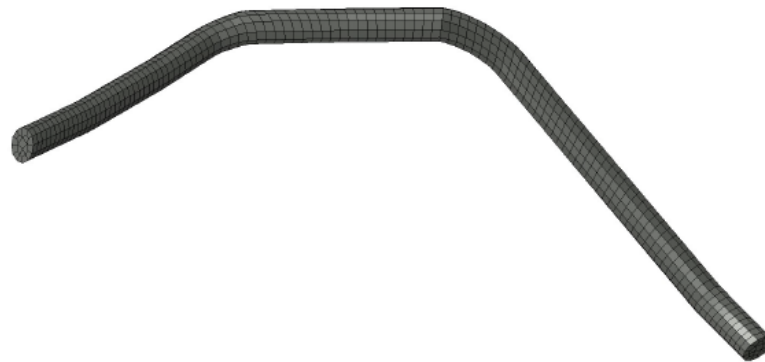
Figure 3.12: Finite element mesh of the CTN, medial view.
