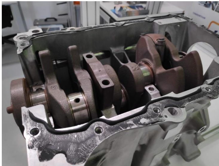
Figure 36. Successful assembly of the bearing cap in its actual working position
