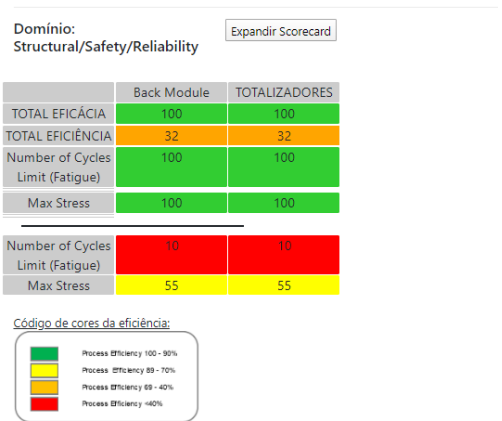
(b) Structural/Safety/Reliability scorecard for iteration 1.4 Back Module
