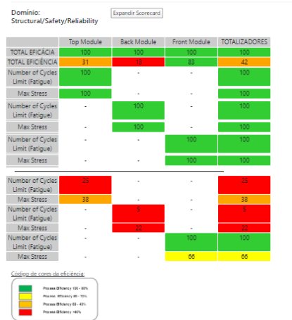
(a) Structural/Safety/Reliability scorecard for iteration 1.1
