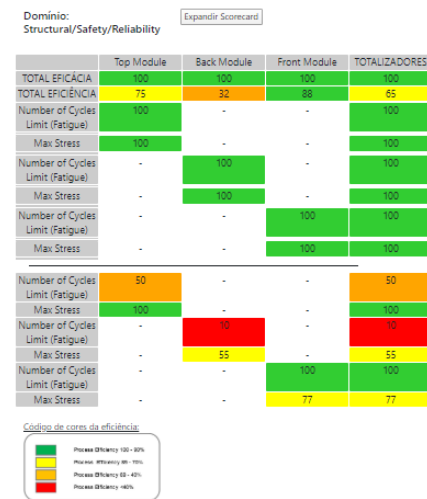
(b) Structural/Safety/Reliability scorecard for iteration 1.4 overall structure
