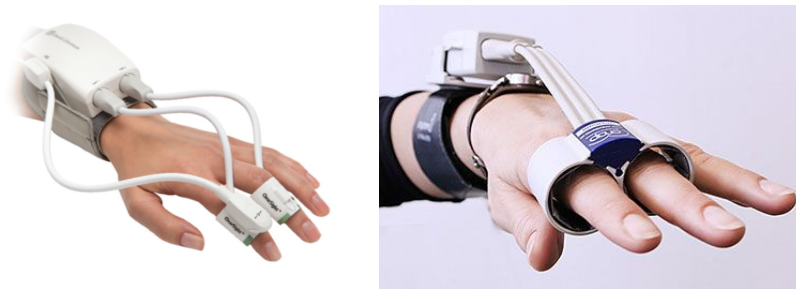
Figure 2.5: Non-invasive continuous blood pressure measuring techniques: ClearSight System 4 (left) and CNAP ® monitor 5 (right).
