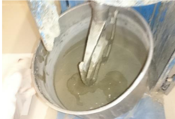
Figure 41. Mixing process in the stage of adding superplasticizer
