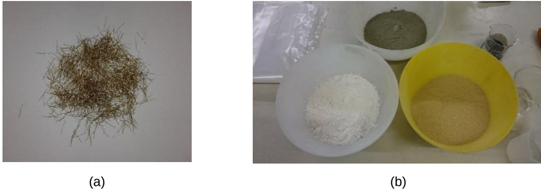
Figure 40. Straight Krampharex fibres with 6 mm length and cross section diameter of 0.175 mm (a). All the material used in the mixture (b).
