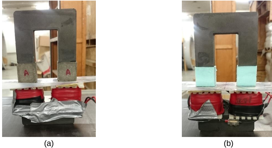
Figure 50. Inductance measurements in cubes (a). Inductance measurement of air ( L_{\text{air}} ) (b).
