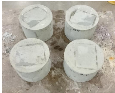
Figure 81. Specimens demoulded 24 hours after casting.
