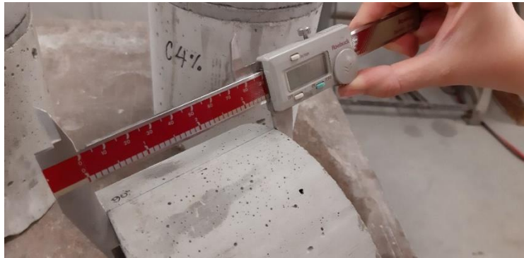
Figure 84. Process of measuring height in specimens.
