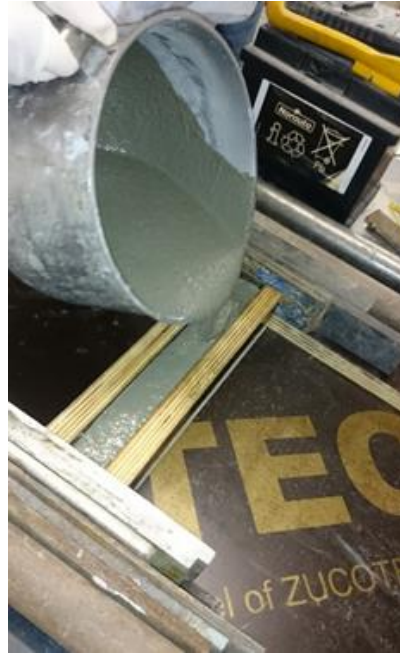
Figure 44. Casting oriented specimens inside fibre orientation set-up.
