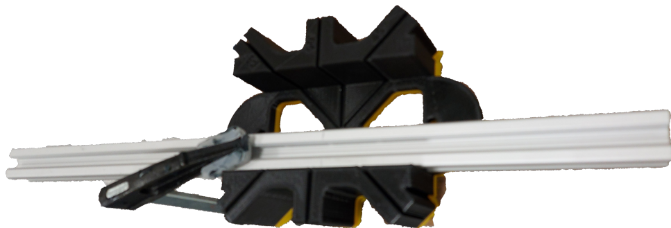
Figure 7.12: Jig created to facilitate manual sawing
