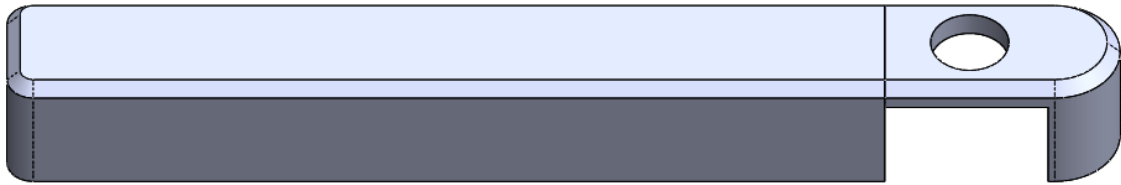
Figure 7.11: Jig created to facilitate assembly
