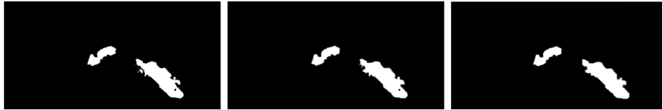
Figure 3.21: Prediction (left); Morphology opening (centre); Morphological closing (right).
