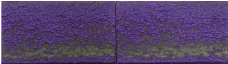
Figure C.9: Fatigue failure surfaces.
