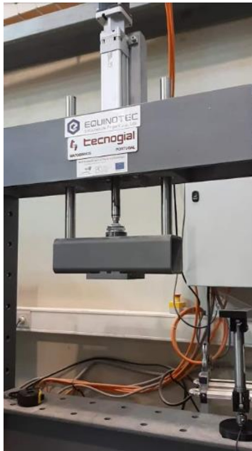
Figure 14 – Equipment that applies sinusoidal force
