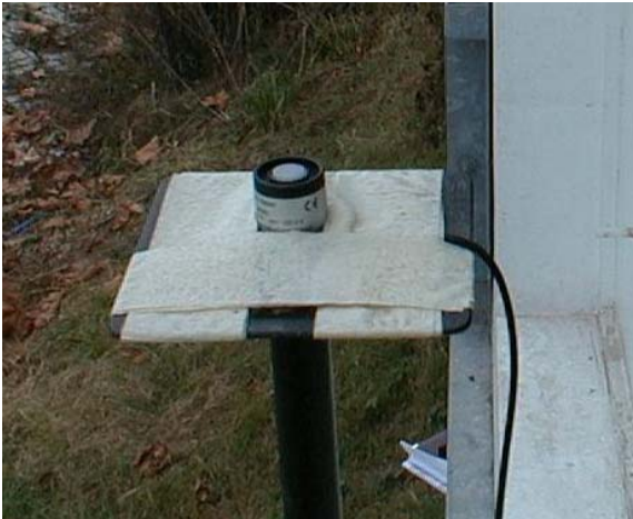
Figure 3-10: Type A luxmeter measuring outdoor illuminance.
