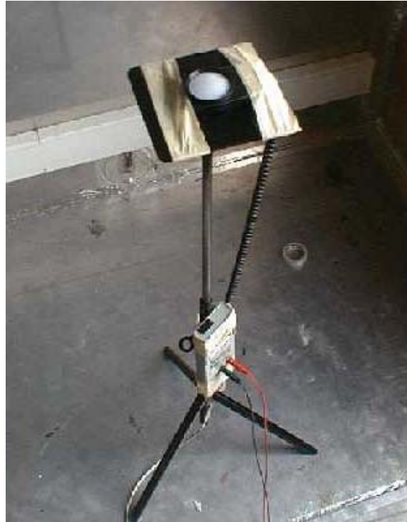
Figure 3-11: Type B luxmeter mounted in the platform.
