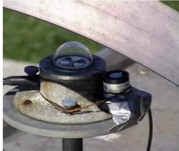
Figure 3-19: Luxmeter attached to pyranometer for measuring outdoor diffuse illuminance
