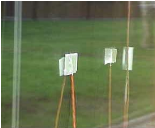
Figure 3-7: Tape protecting glazing temperature sensors from direct radiation.
