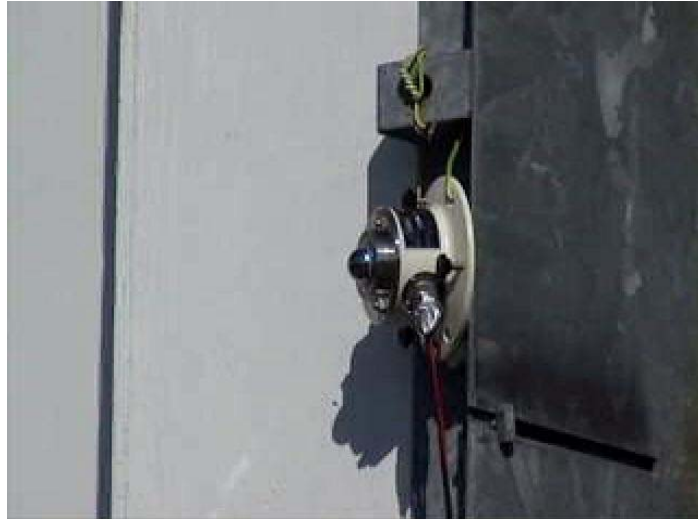
Figure 3-20: Pyrgeometer for measuring the LW radiation impingent at the external surface of the glazing.
