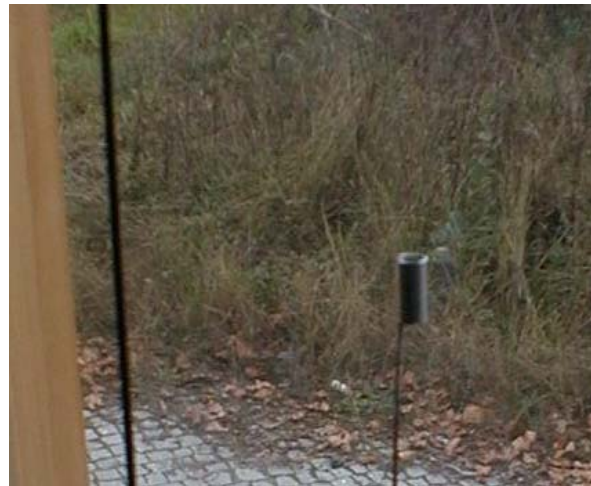
Figure 3-8: Cylinders protecting air temperature sensors from direct radiation.
