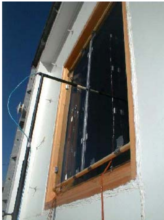
Figure 3-5: A view of the Solvent window prototype mounted in Summer mode.
