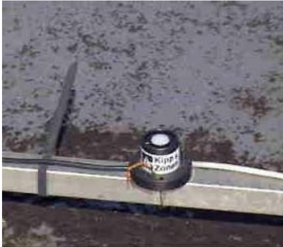
Figure 3-18: Luxmeter for measuring outdoor global illuminance
