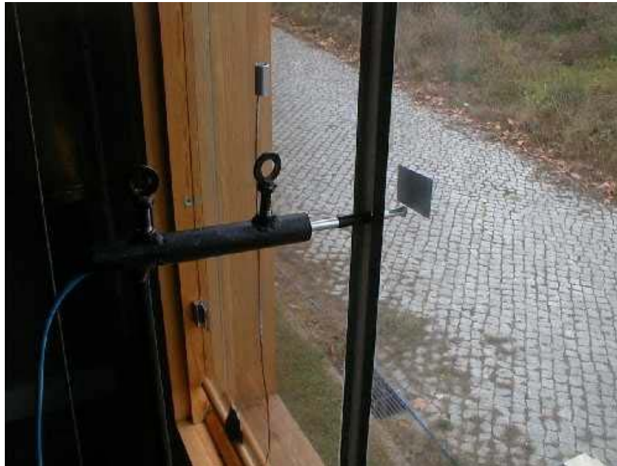
Figure 3-12: Hot-wire anemometer insertion in the air gap during the first measuring campaign, here in Winter mode.
