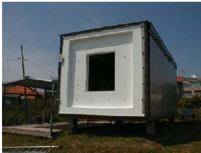
Figure 3-2: A view of the PASSYS test cell with the aperture for the test component in the South façade.
