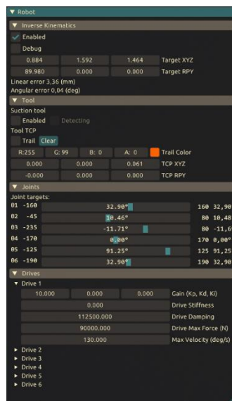
Figura 3.6 - Painel “Robot” e as suas quatro partes: “Inverse Kinematics”, “Tool”, “Joints” e “Drives”
