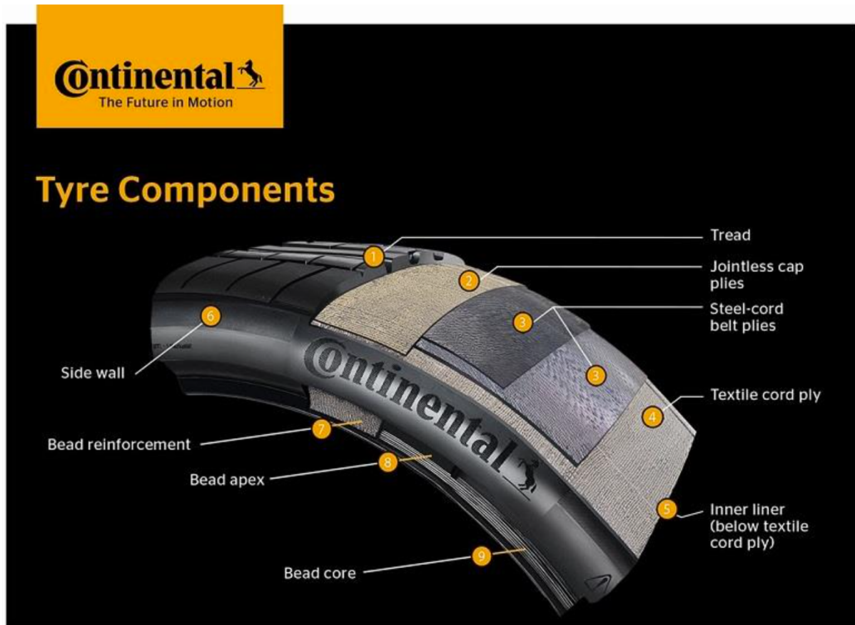
Figure 2 -Example of tire constitution (adapted from Continental, 2019).
