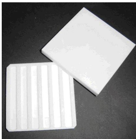
Figure 13. Teflon mould for samples preparation.
