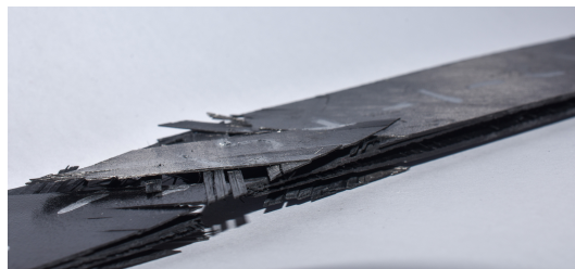
Figure 5.5: Delamination detail on a post-mortem H2 plain strength tension specimen.
