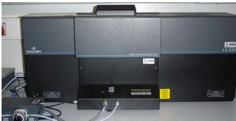
Figura 35: Coulter – LS Particle Size Analyzer.
