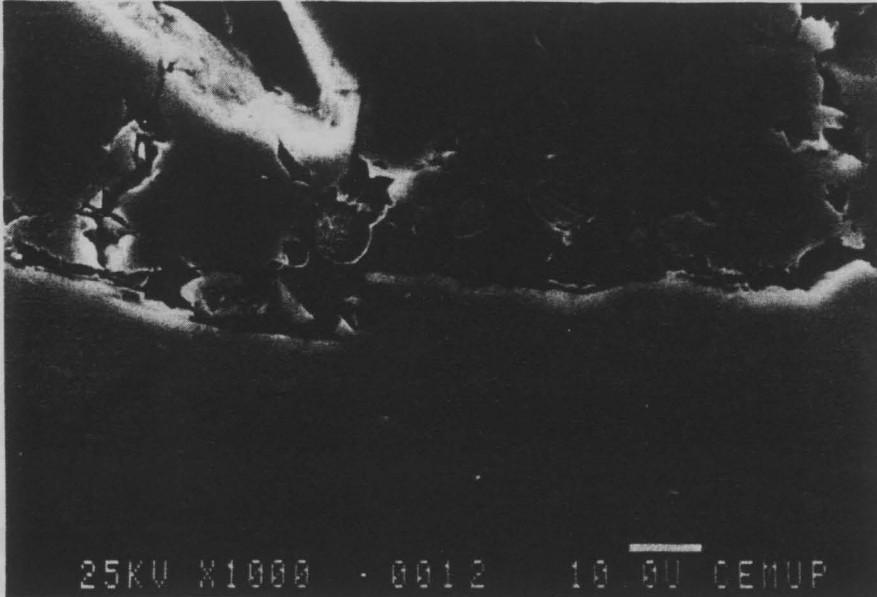
Fig.5- Cross-section of a plasma-sprayed sample showing cracking and large pores in the coating layer.
