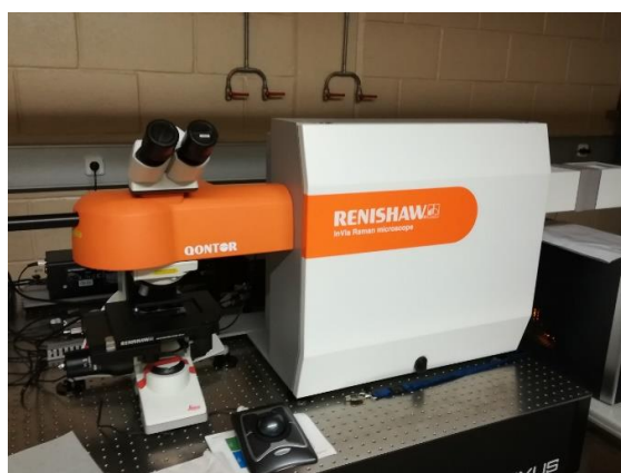
Figure 4. Experimental setup utilised for present work, in first plane the inVia Qontor Renishaw confocal Raman spectrometer. In the background the set of lasers available: 532 nm, 633 nm and 785 nm.
