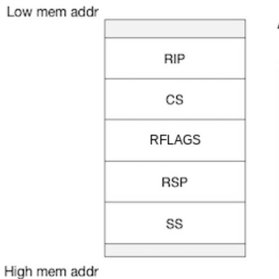
Figure 3.1: Expected stack frame layout at the time of an iret instruction [60]
