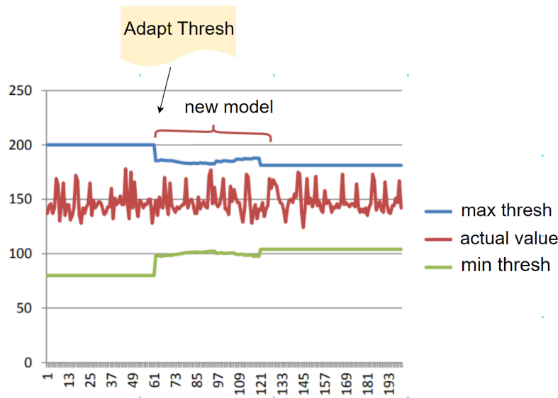
Figure 5.28: Example of a Belt Position Acceptance Thresholds Adjustment (pixels), when a new model is produced [152, 213].
