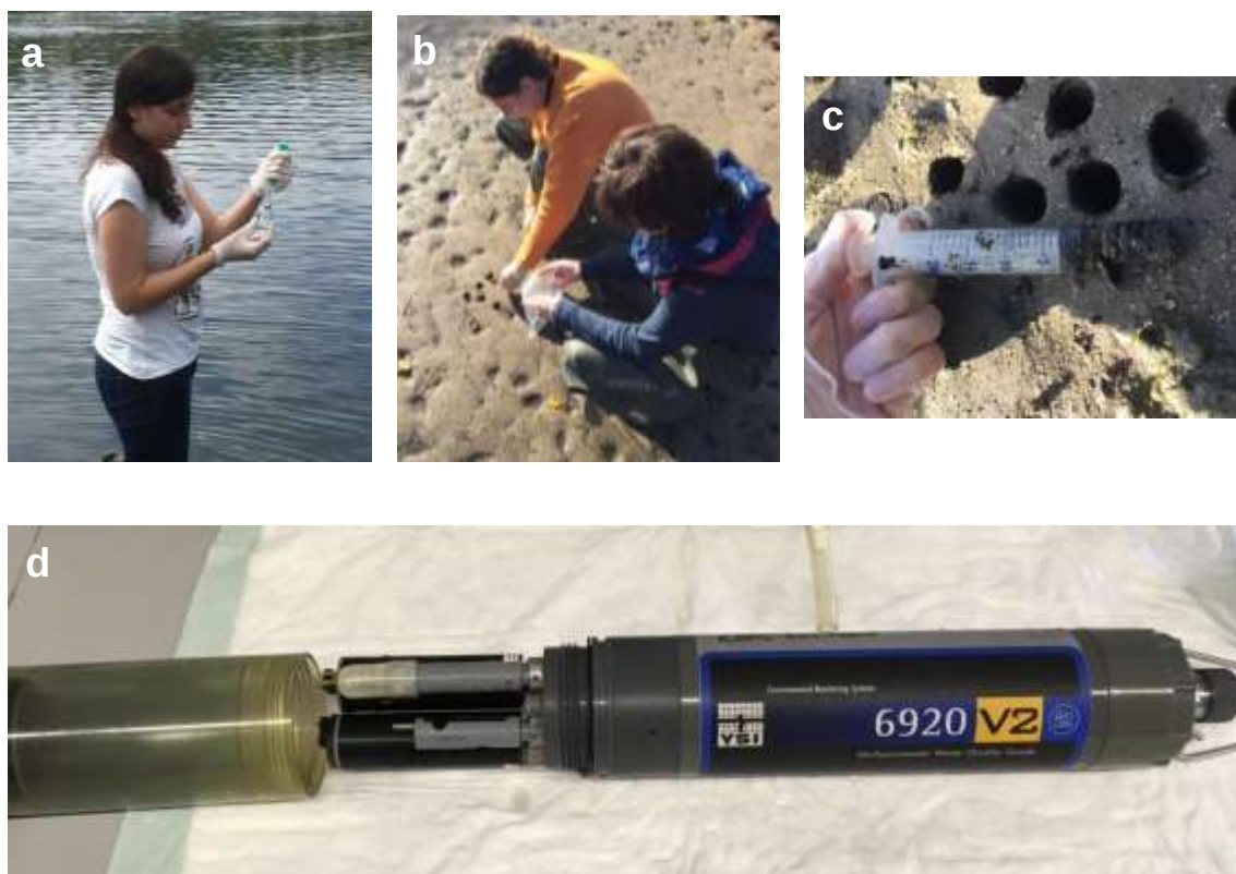
Figure 5 –Sampling collection (water collection (a), sediments collection (b, c)), and multiparametric sonde used to measure water variables in situ (d).
