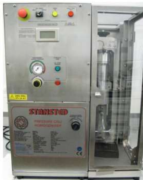
Figure 9 - High pressure homogenizer used to prepare the lipid nanoparticles. SPCH-10, Stansted Fluid Power, UK.
