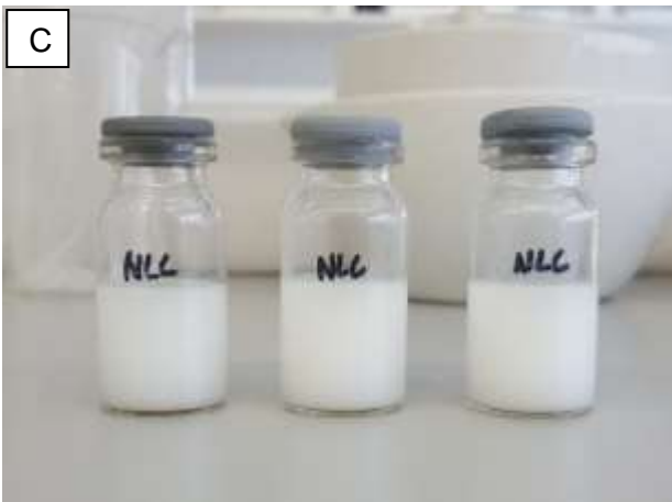
Figure 59 – Aspect of unloaded NLC dispersions prepared by ultrasonication (A) after their preparation and after (B) 30 and (C) 60 days of storage at 4 °C.
