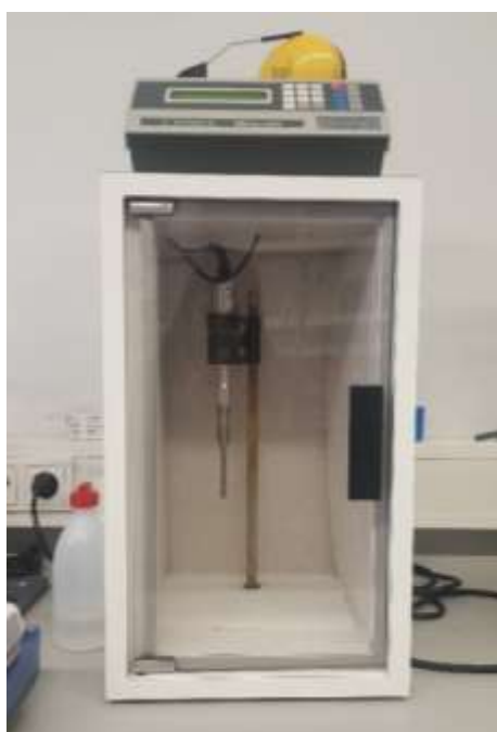
Figure 10 – Ultrasonicator used to prepare the lipid nanoparticles. VibraCell VCX130, Sonics & Materials Inc, USA.
