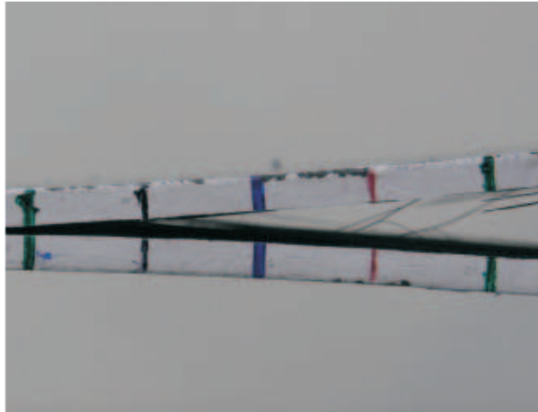
Figure 2-17: Fibre bridging in a DCB test specimen.
