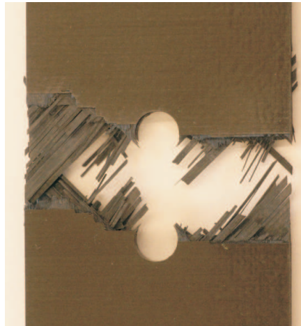
Figure 5-12: Net-section failure in an open-hole specimen.
