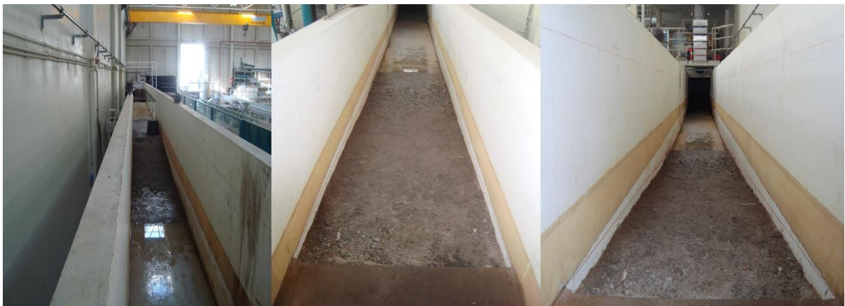
Figure 3.4 - Stage 1: Breaking of 0.29 m of the ground thickness.
