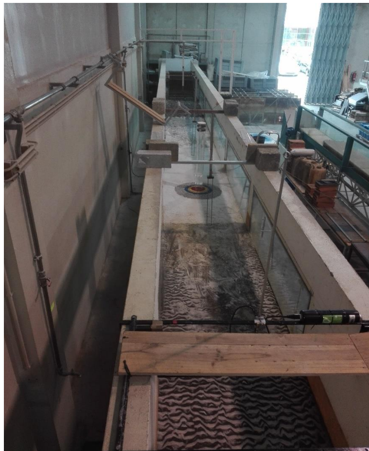
Figure 3.58 - Final layout of the flume with the model ready to test.
