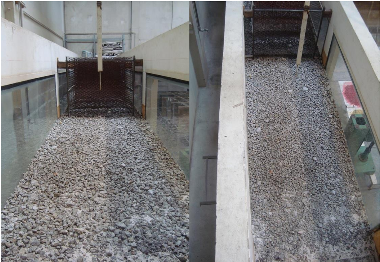
Figure 3.52 - Rock mattress (front and top view).
