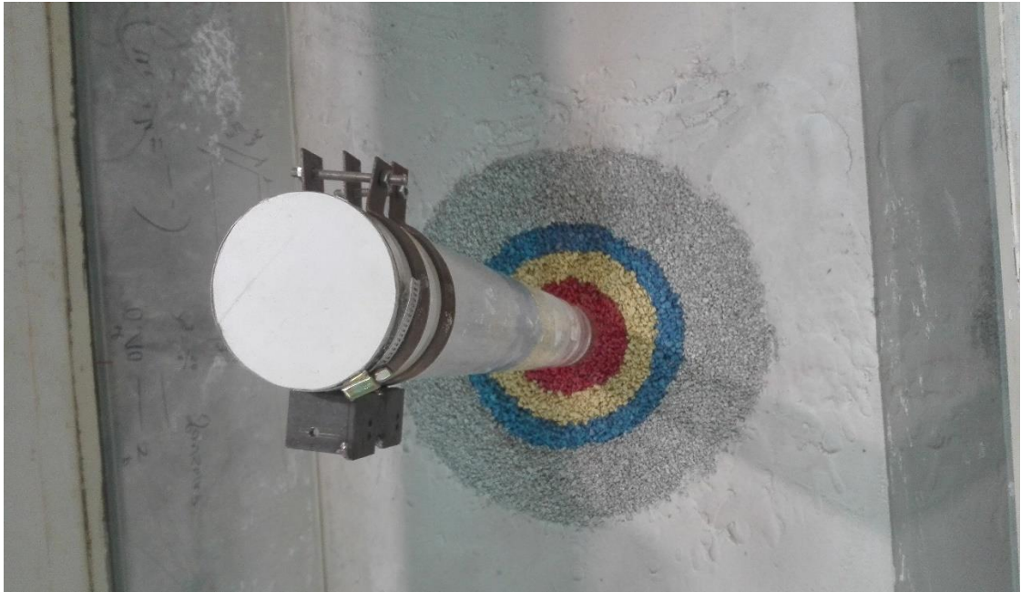
Figure 3.57 - Top View of the monopile model.
