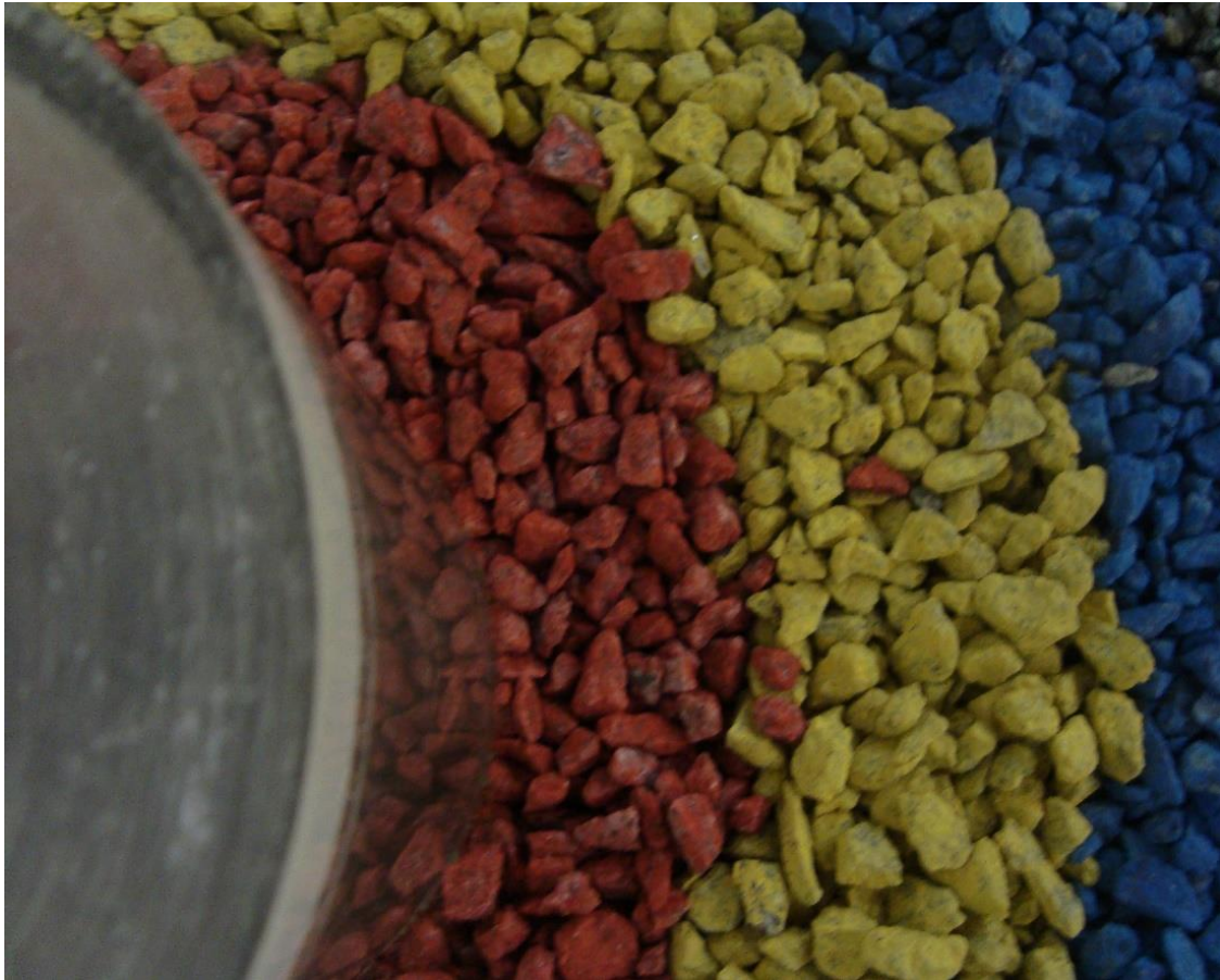
Figure 4.23 - Stone movement for 5000 waves (zone 1).
