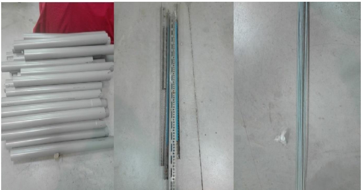
Figure 3.12 – By-pass boxes materials (PVC PN6 \Phi=90 mm pipes; L60/40 galvanized steel profiles; Threaded \Phi=5 mm stainless steel rods).
