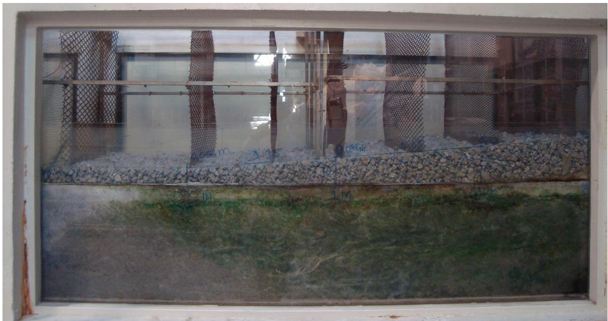
Figure 3.47 - Gravel profile at the dissipation system.
