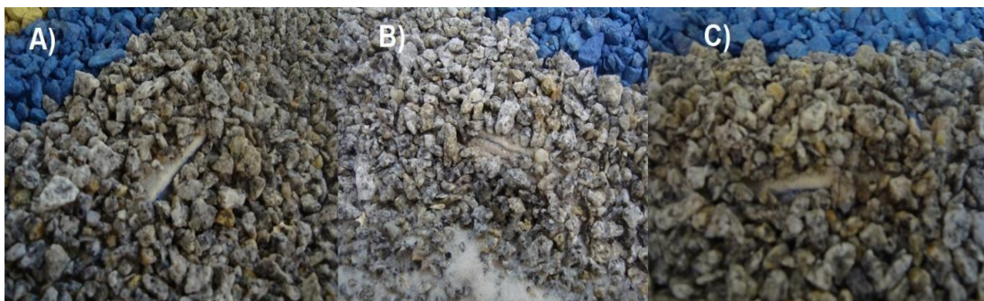
Figure 4.22 - Filter exposures for 5000 waves (A - G1; B - G2; C - G3).
