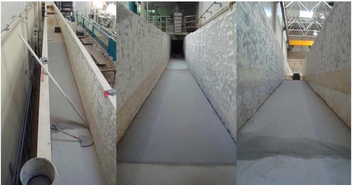
Figure 3.6 - Stage 2: Approach Ramp (5.8 m long with 1/20 slope).
