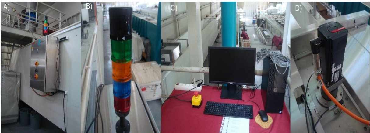
Figure 3.22 – Wavemaker main electrical elements: (a) MDCP; b) Light Beacon; c) Wave generating computer and Remote Paddle Safety Unit; c) Low Inertia AC servo Motor.
