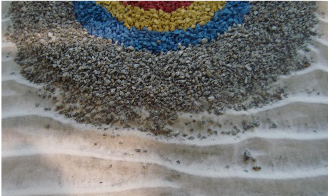
Figure 4.36 - Bottom edge after 9000 waves.
