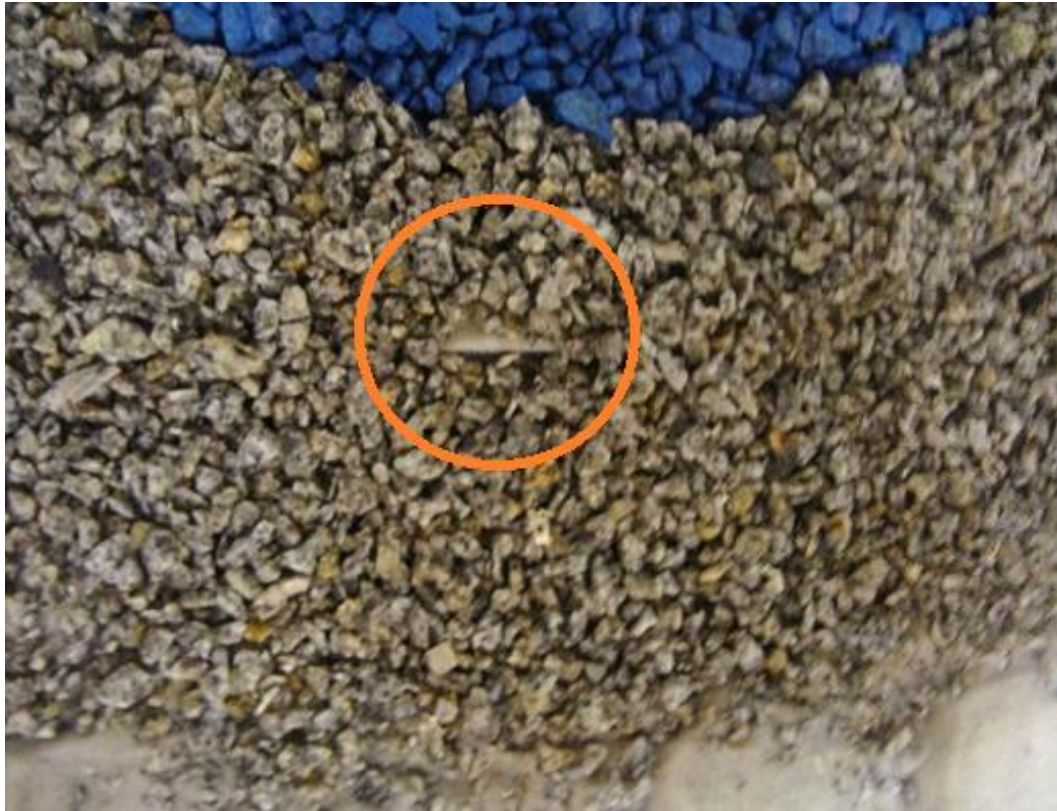
Figure 4.20 - Filter exposure (G1) for 3000 waves in the Test 1b.
