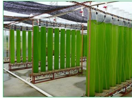
Figure 2. 4 - Vertical column PBR (Adapted from: Huo et al. 2018).
