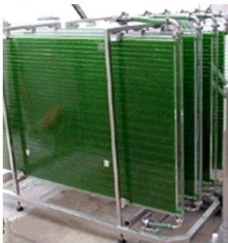
Figure 2. 5 - Flat-plate PBR (Adapted from: Ojamae 2019).
