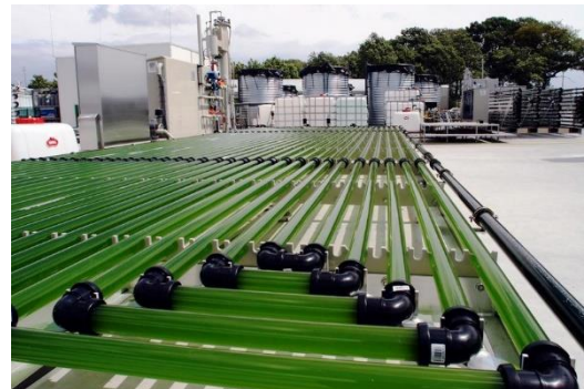
Figure 2. 6 - Horizontal tubular PBR (Adapted from: Climate-Kic 2019).
