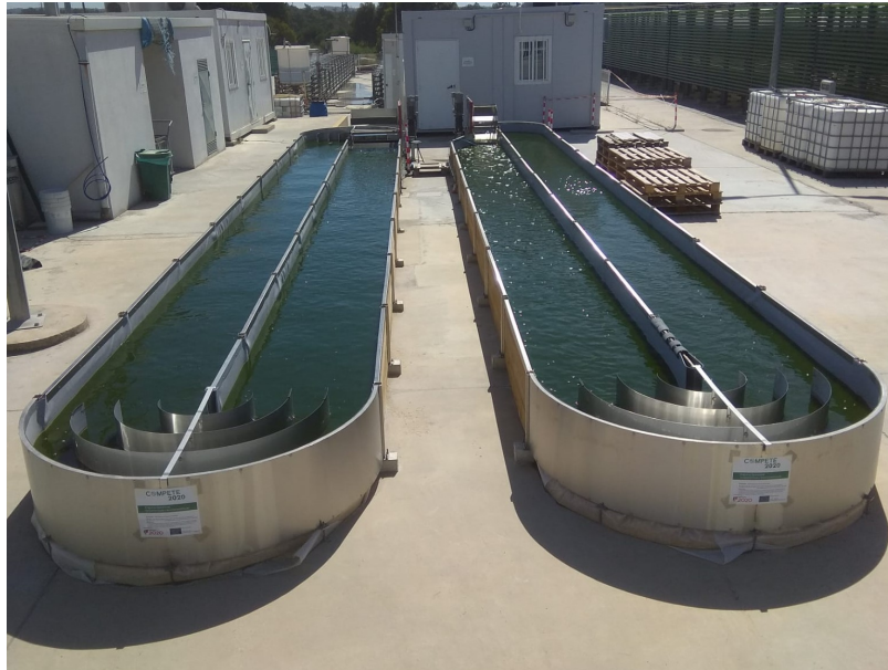
Figure 5. Pilot-scale raceway ponds used in these study. Modified raceway at right and standard raceway at left.
