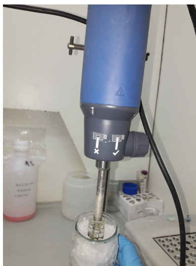
Figure 8. Biomass homogenization by cell breakdown.
