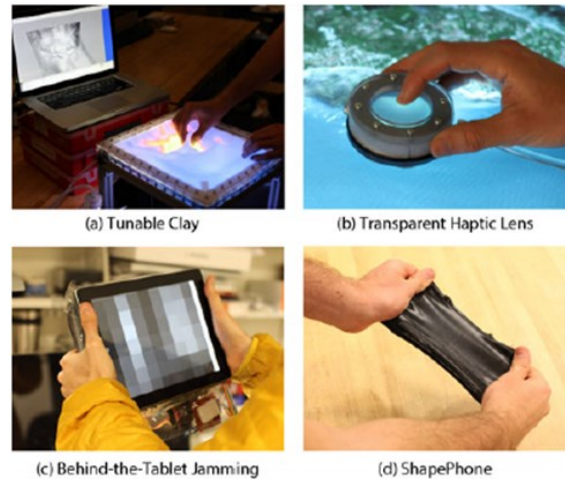
Figure 4 - Four examples of Haptic devices based on particle jamming [8]
