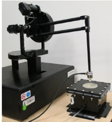
Figure 12 - Experimental test set-up using the Phantom Premium haptic device [20]
