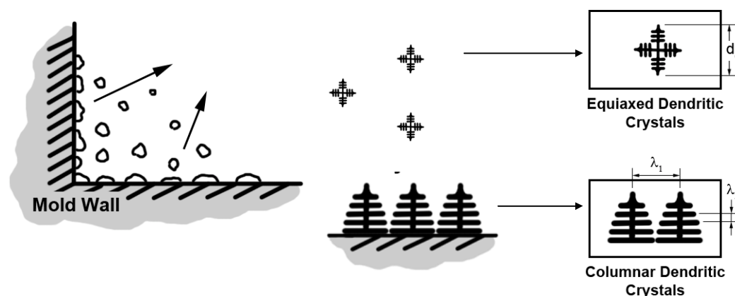
Figure 2.23: Solidification structure found in the mould wall interface.
