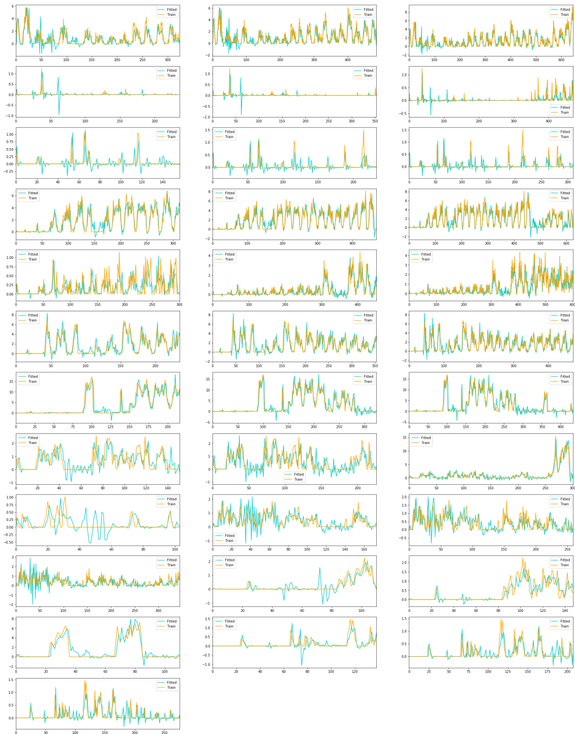
Figure B.1: Training values (orange) versus fitted values (blue) by ARIMA(6, 1, 2)(2, 1, 0)_{24} considering all folds
