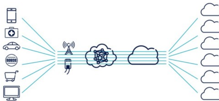
Figure 2.3: Network Slicing visualised.
