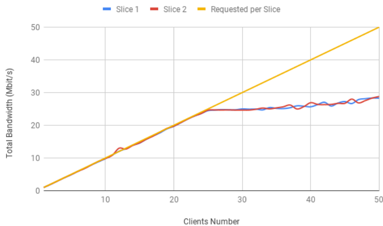
Figure 4.14: Two slices policing implementation total bandwidth.
