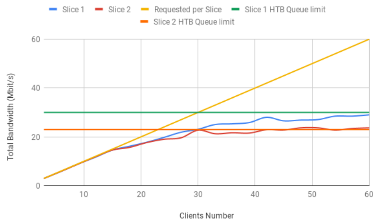
Figure 4.35: Two slices DSCP matching with prioritisation - Both slices total bandwidth.
