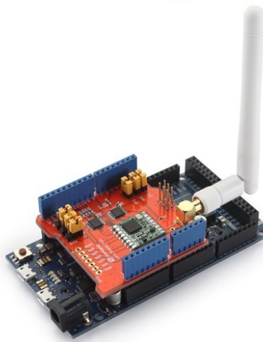
Figure 3.5: Dragino LoRa shield used as access point.
