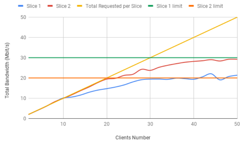
Figure 4.29: Two slices DSCP marking - Total achieved bandwidth in each slice.
