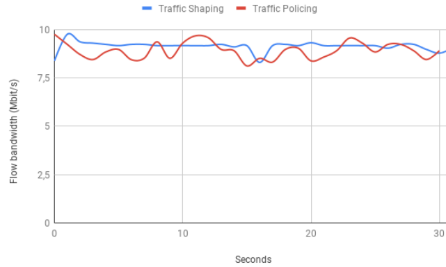
Figure 4.13: Server perspective UDP flows on traffic policing and traffic shaping.
