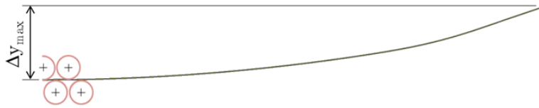
Figure 3.13 – Maximum vertical displacement measurement procedure.
