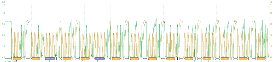
Figure 6.3: I 2 C SDA and SCL signals 50 meter UTP bus
