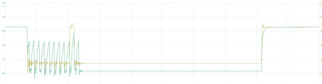
Figure 6.4: I 2 C SDA and SCL signals - 70 meter UTP bus
