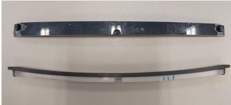
Figure 46: Combiner samples cut horizontally after the polishing process
