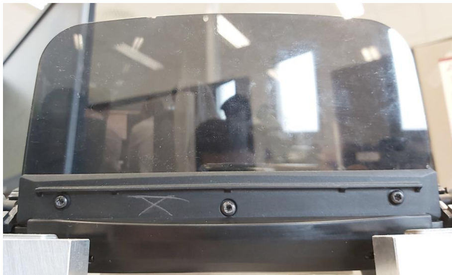
Figure 13: BMW Combiner Unit
