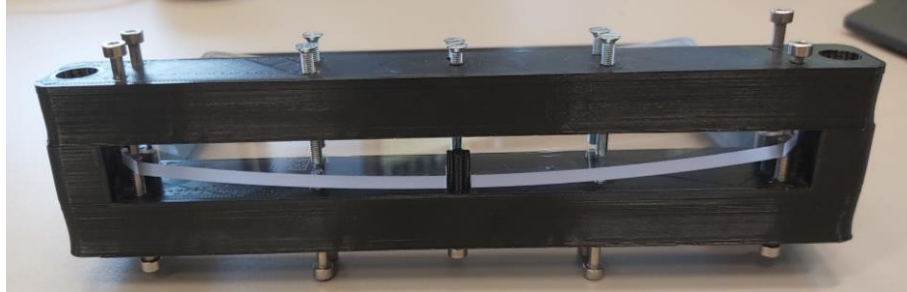
Figure 83: Mounted and tightened combiner
