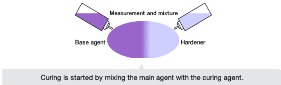
Figure 23: Two-part epoxy curing process. (ThreeBond, 2019)
