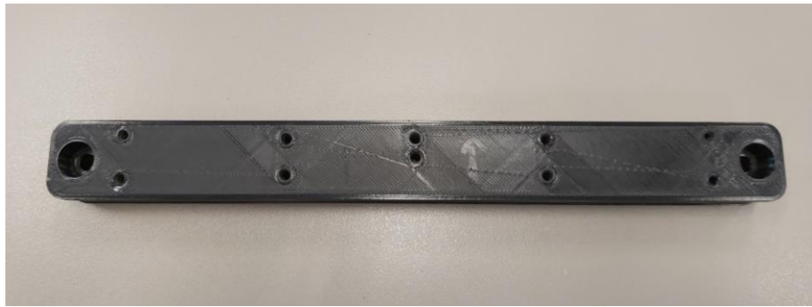
Figure 81: Top part of the jig
