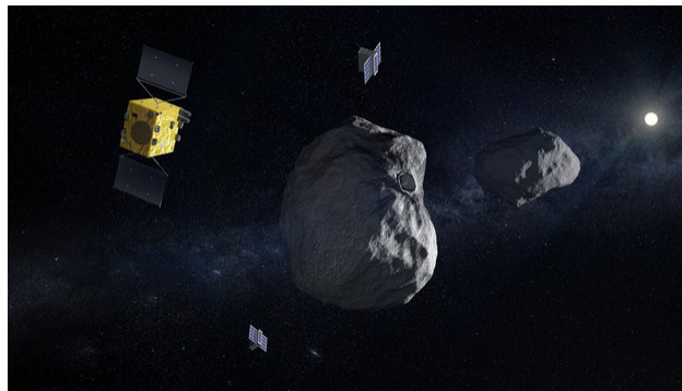
Figure 2.8: Hera mission concept. Mother-ship orbits the asteroid system alongside APEX and Juventas CubeSats [75].
